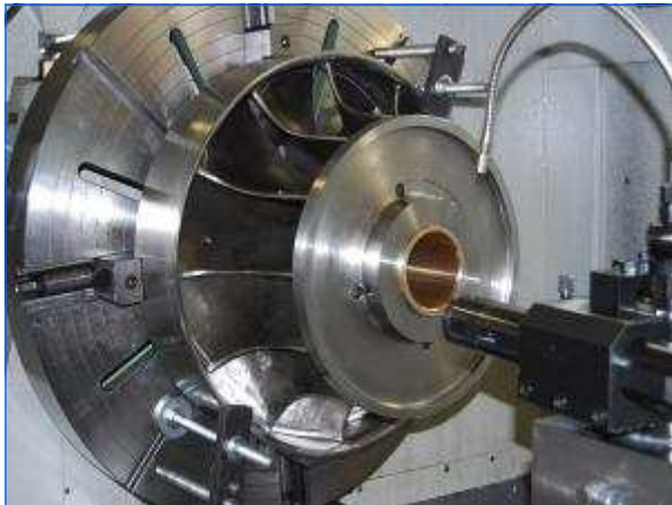
Fertigung Francis Laufrad Manufacturing of the francis runner
