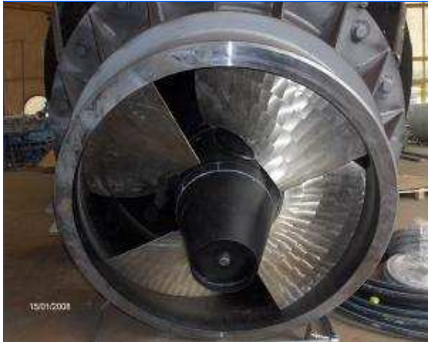
Kaplan Laufrad in Laufradring eingebaut Kaplan runner fitted in runner ring
