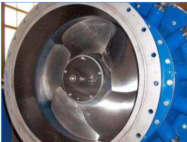
Lauftradmontage in der HYDRO ENERGY Montagehalle Runner assembly in the HYDRO ENERGY workshop
