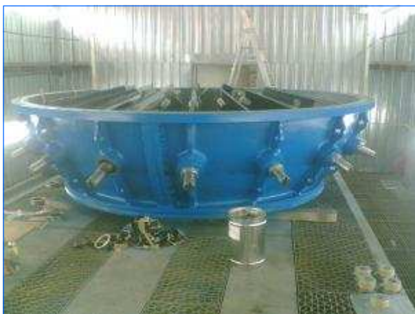
Leitapparat bei Endmontage Control device at final assembly
