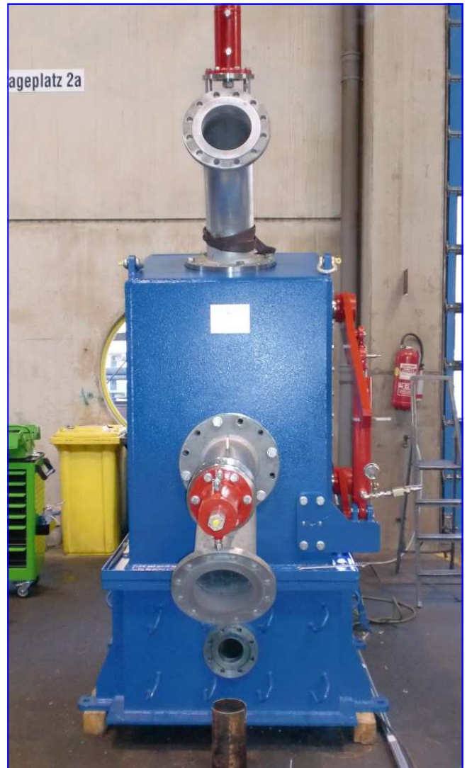
Pelton Turbine Pelton turbine
