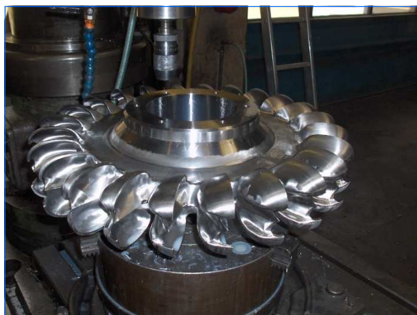
Peltonlaufrad Endbearbeitung Pelton runner finishing operation
