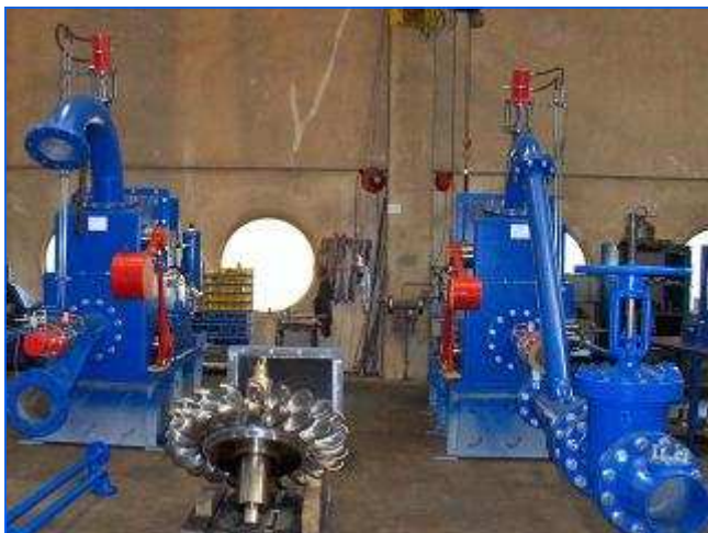
Beide Pelton Turbinen vor Auslieferung Both Pelton Turbines before delivery
